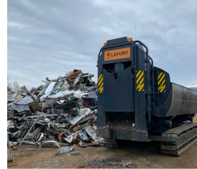
TRAX650 from Peacock's Recycling has a 6-meter box (19'8"), a pusher force of 180 tons (200 US), two wrap-around wings of 240 t (265 US) and a diesel engine of 302 HP.
