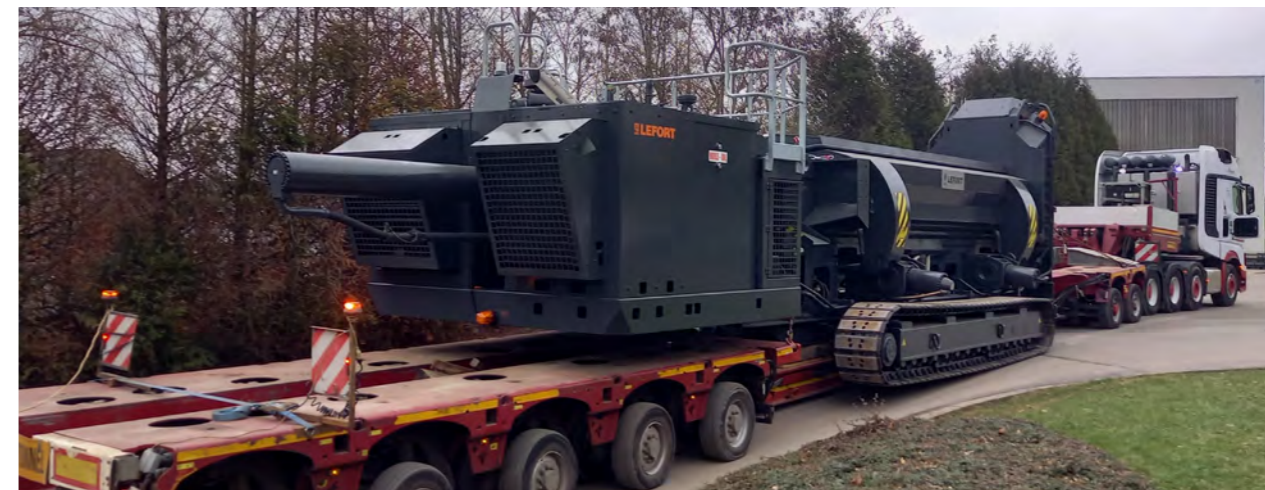
LEFORT TRAX 700 scrap shear at Bader Recycling: cutting force 700t, compression box 6600x2600 mm, hold-down 120t, pusher 180t, press force on each wing 325t, diesel engine of 400 hp.
