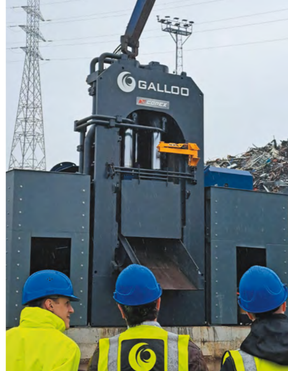
New LIDEX at GALLOO: cutting force of 2,000 tonnes, large blade width of 1,500 mm, 10-metre box and powerful 8x110 kW hydraulics
