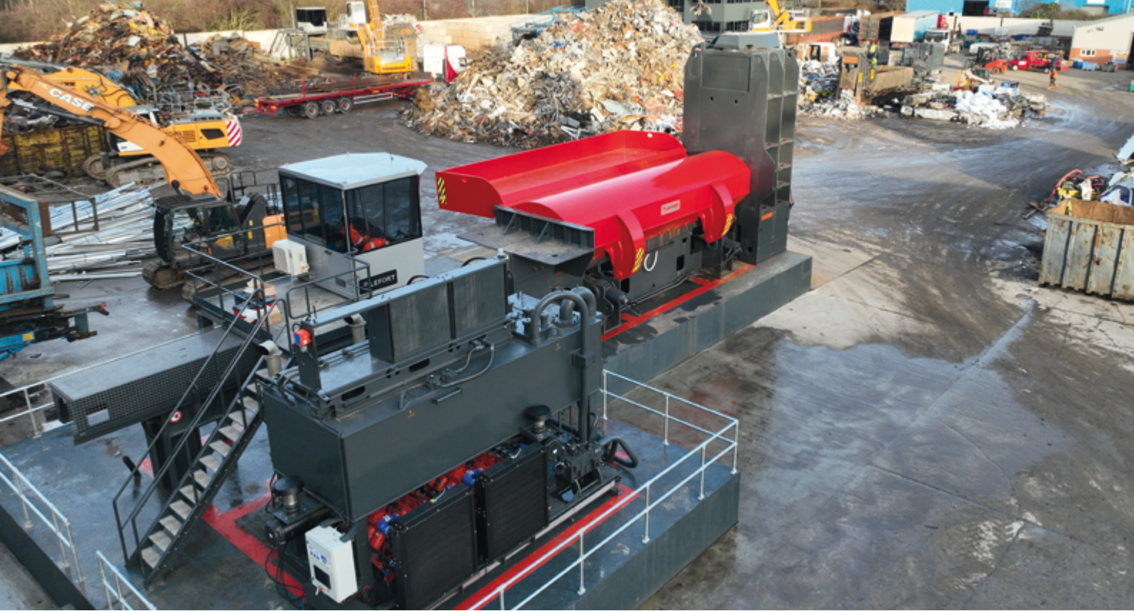
KOLOSS by Northern Metal Recycling – 1,450 tonnes of cutting force, powered by a powerful Scania V8 diesel drive, with an 8-meter box and a loading hopper.
