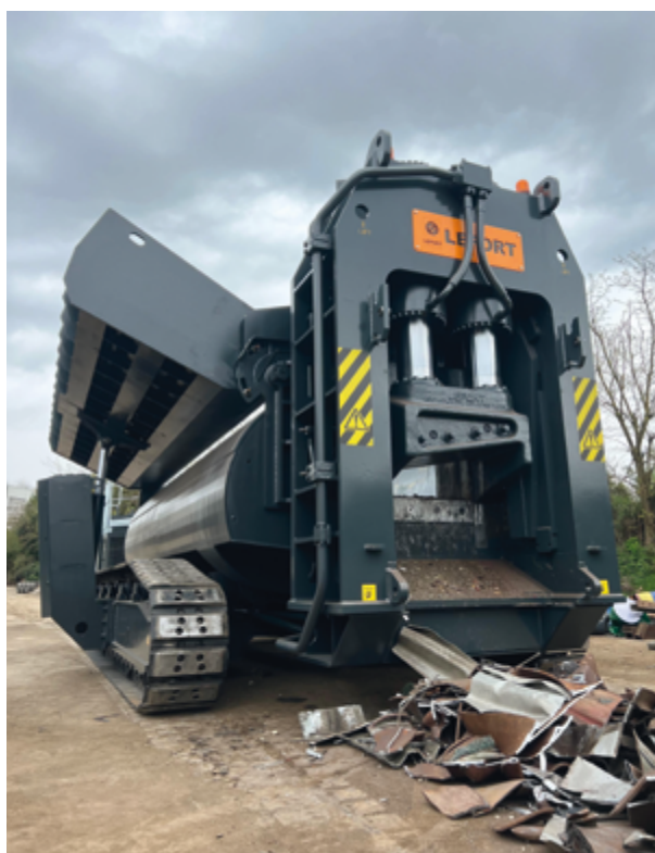
The TRAX, one of LEFORT®'s flagship products, combines mobility and productivity, offering operators greater flexibility in their day-to-day operations. Here, a 1,250-ton cutting force (1,375 US tons) version with a loading table, installed at OmniSource, LLC in Indiana.
